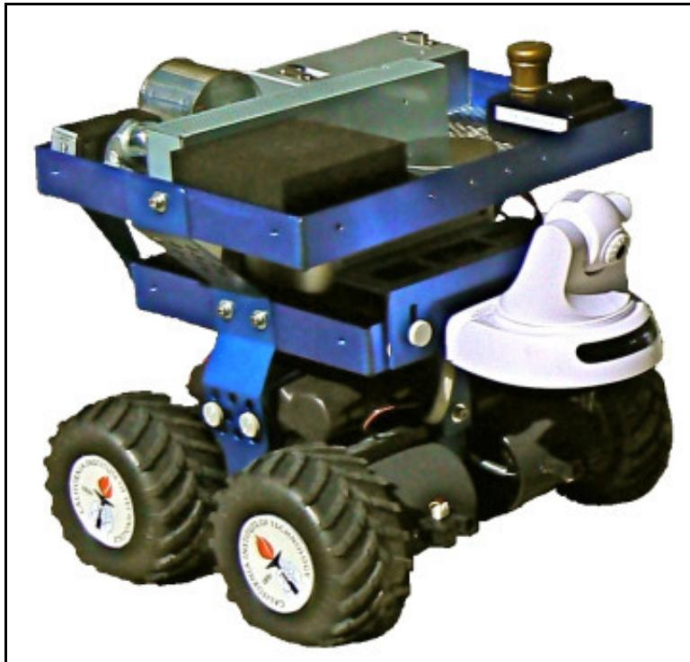
*Cyclops is an all-wheel-drive platform that could enhance the design of visual prostheses and be adapted for autonomous planetary exploration.*
