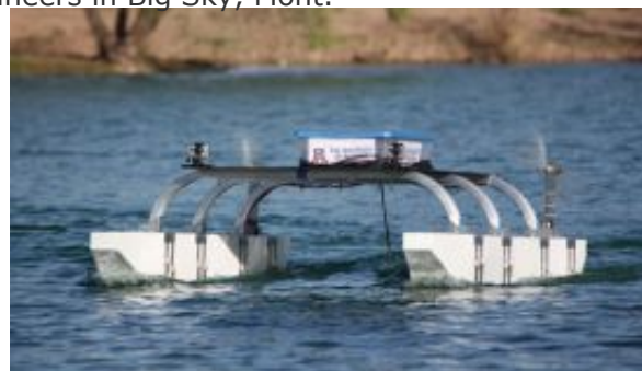
The lake lander TEX II is the latest component of Wolfgang Fink's autonomous planetary exploration fleet.
