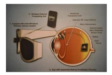
An overview of the retinal implant that uses the processing unit or iPhone/iPod to capture and process images and then transmit the information to an implanted microelectronic system. The implant decodes the data and stimulates the retina with a pattern of electrical impulses to produce visual perceptions. Illustration provided by Dr. Wolfgang Fink
