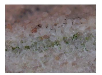
Finally, the same imager would be used to take pictures on a microscopic level. Here, the modified camera revealed green biomass thriving between mineral grains in a rock. (Photo: Wolfgang Fink)
